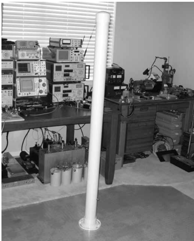
Figure 18 – Completed 1296 MHz helical collinear prototype
