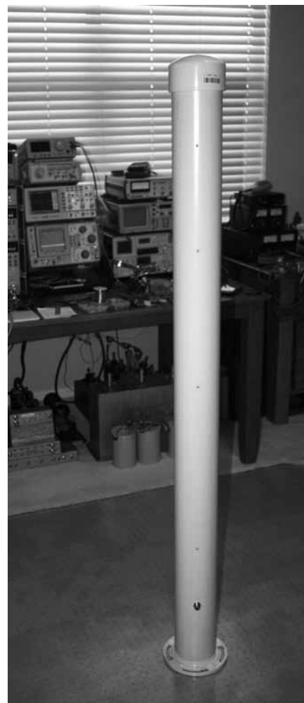
Figure 15 – Completed 902 MHz helical collinear prototype
